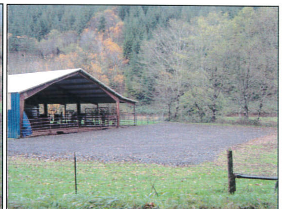
Before/After photos: 5000 square feet of grading, fabric and rock added as protection to muddy heavy use area on ranch adjacent to Big Elk Creek. Reduces sediment and bacteria to creek.
